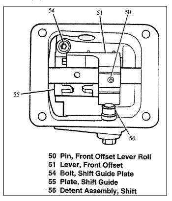
Figure 2-9. Shift Detent Assembly.
