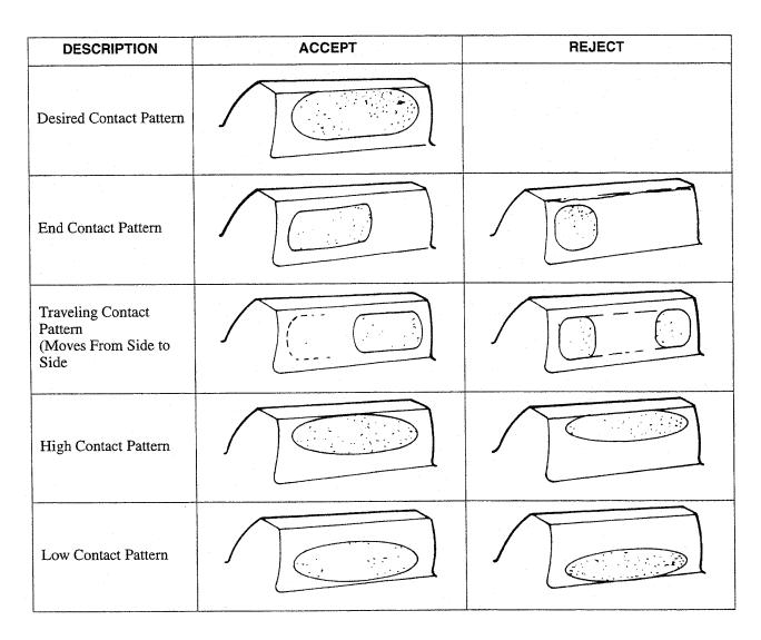
Figure 3-2. Gear Tooth Contact Patterns
