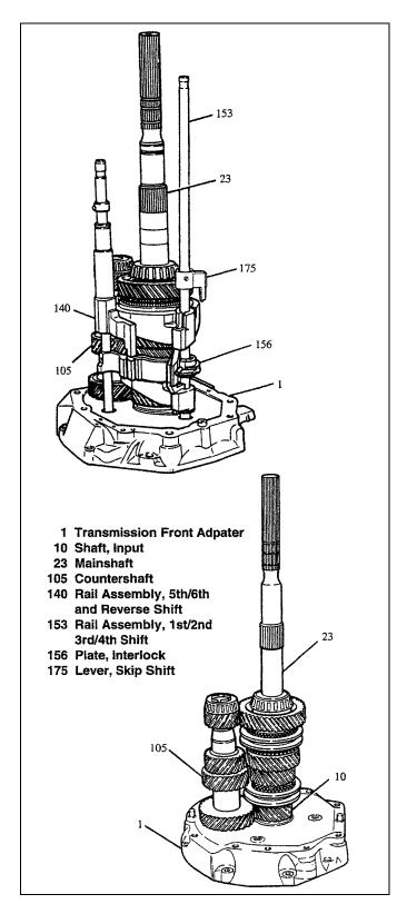
Figure 4-1. Shift Rail Assemblies and Gear Clusters
