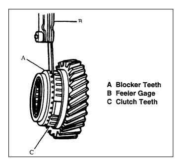
Figure 3-13. Measuring blocker Ring Wear.
