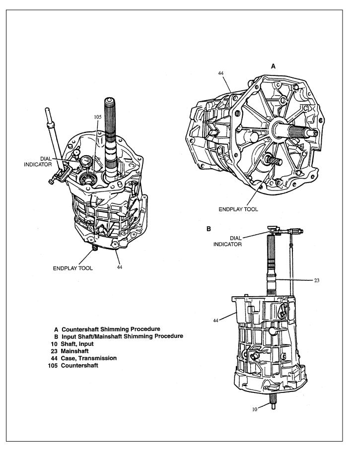
Figure 5-1. Input Shaft, Mainshaft and Countershaft Shimming Procedure
