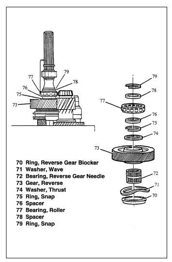
Figure 2-5. Reverse Speed Gear
