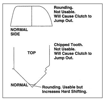
Figure 3-3. Clutch Tooth Inspection
