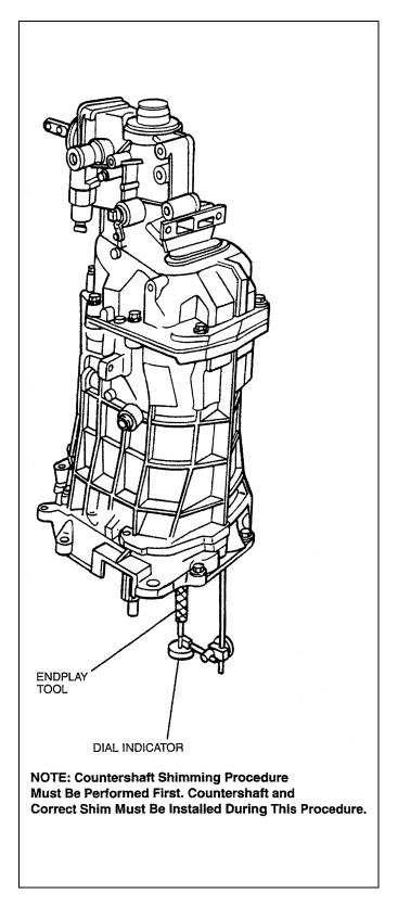
Figure 5-2. Countershaft Extension Shimming Procedure
