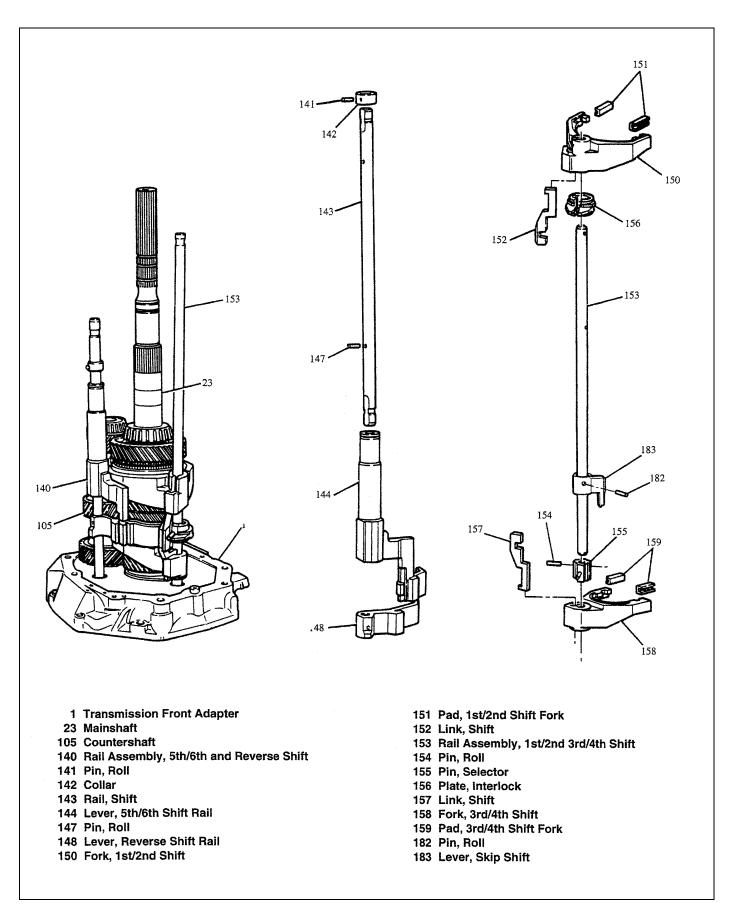
Figure 3-14. Shift Rail and Fork Assemblies
