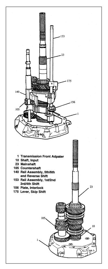
Figure 2-11. Shift Rail Assembly and Gear Clusters
