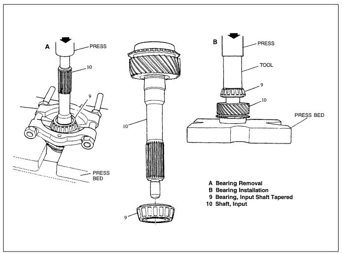
Figure 3-5. Input Shaft
