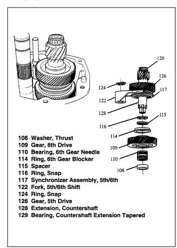
Figure 2-8. Countershaft Extension Assembly
