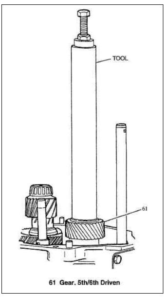
Figure 4-4. 5th/6th Driven Gear
