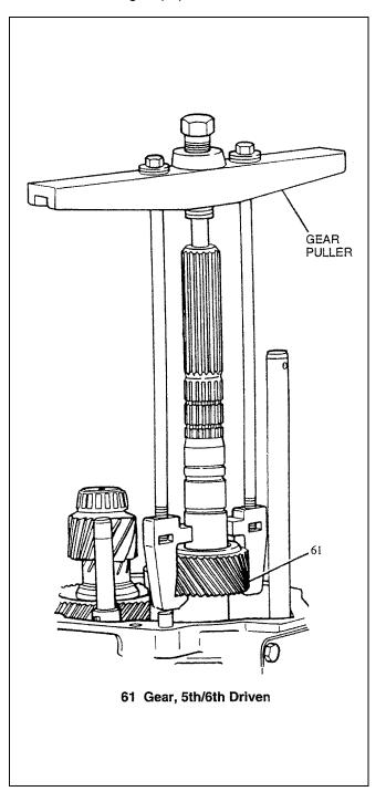
Figure 2-7. 5th/6th Driven Gear
