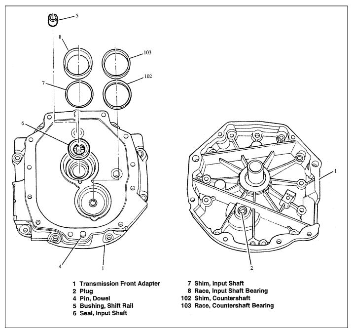
Figure 3-15. Transmission Front Adapter
