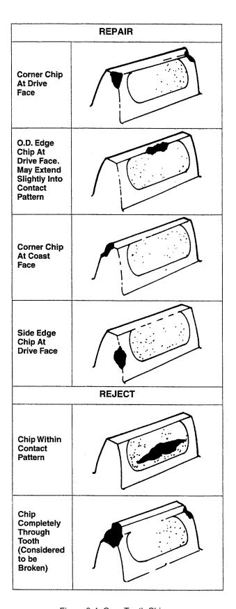
Figure 3-4. Gear Tooth Chips
