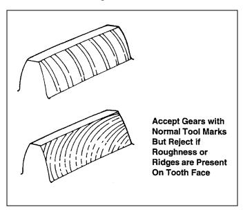
Figure 3-1. Normal Gear Tooth Tool Marks
