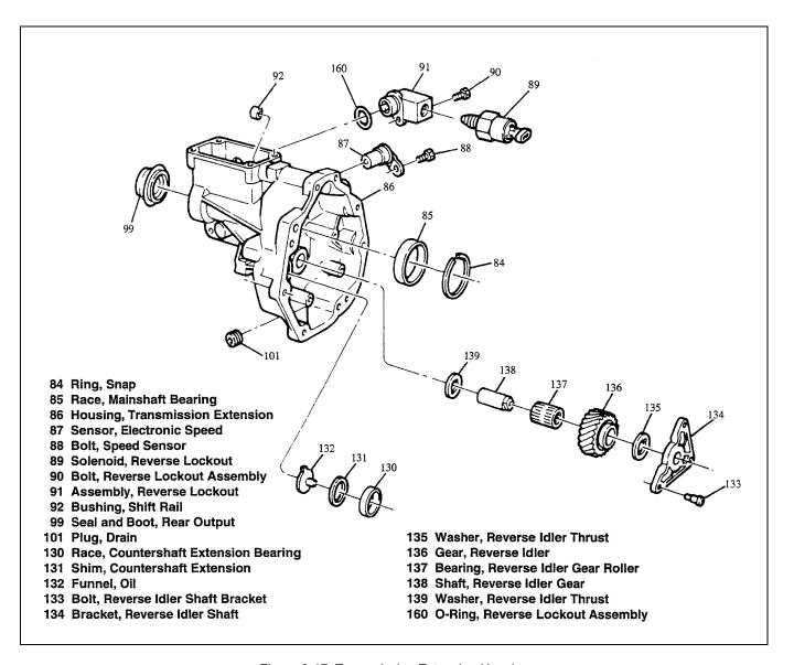
Figure 3-17. Transmission Extension Housing
