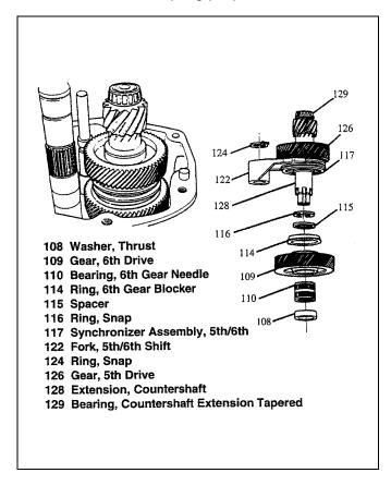
Figure 4-3. Countershaft Extension Assembly.
