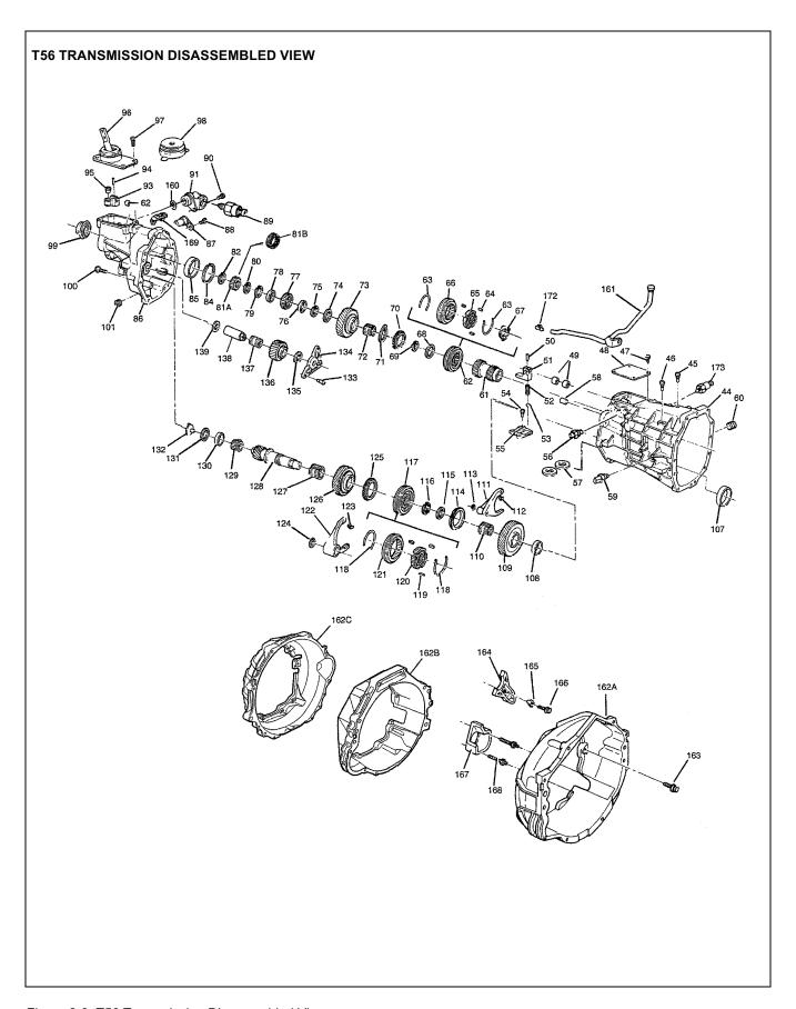
Figure 2-3. T56 Transmission Disassembled View
